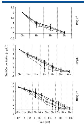
Figure 3. TAN consumption in the reactors fed with TAN concentrations of 2, 5 and 10 mg  $\rm L^{-1}$ .
