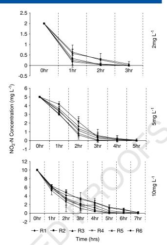
Figure 4.  $NO_2$ -N consumption in the reactors fed with  $NO_2$ -N concentrations of 2, 5 and 10 mg  $L^{-1}$ .
