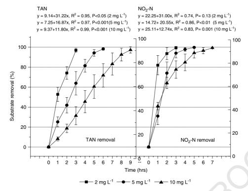
Figure 5. Percentage TAN and  $NO_2$ -N removal rates in the reactor system at initial substrate concentrations of 2, 5 and 10 mg L<sup>-1</sup>.
